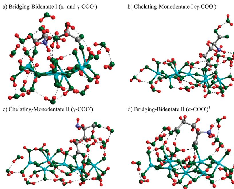
**Figure 6.** Surface speciation models resulting from quantum chemical calculations for aqueous glutamate reacted with the (101) surface of rutile; (†) outer-sphere coordination through  $\gamma\text{-COO}^-$  also present. In all surface species, H-bonding (dashed lines) between carboxyl groups attached to the rutile surface is present for O atoms not covalently bound.
