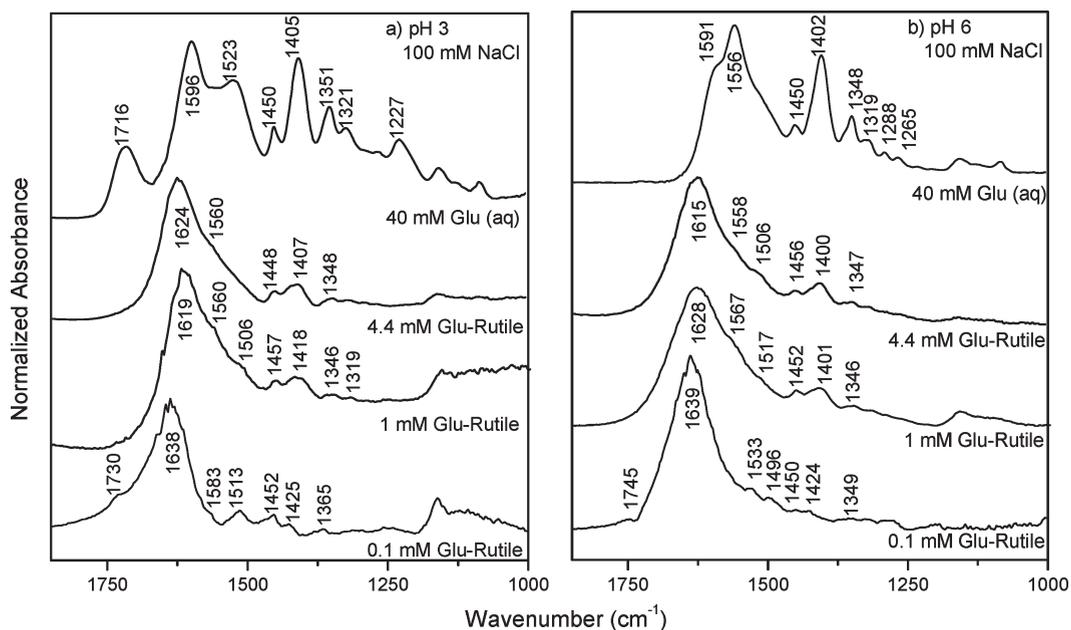
**Figure 5.** ATR-FTIR spectra of glutamate (Glu) adsorbed to rutile films at (a) pH 3 and (b) pH 6 ( $\text{mM} = \text{mmol kg}^{-1}$ ).
