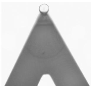
**FIGURE 1.** A modified standard  $\text{Si}_3\text{N}_4$  AFM cantilever with a  $6.8 \mu\text{m}$  silica microsphere attached to the tip.
