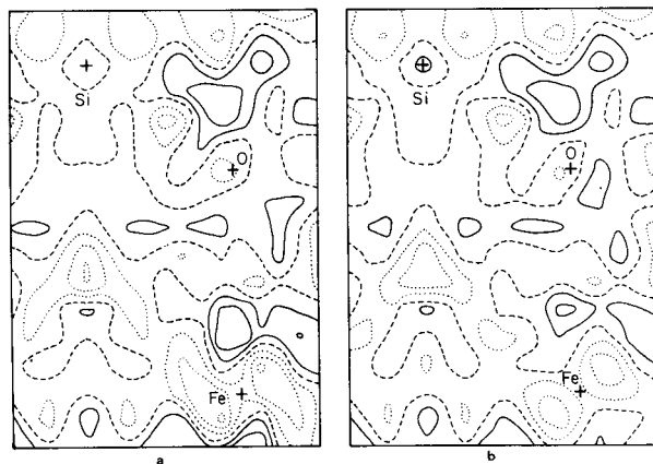
Fig. 3. Partial section of the difference electron density for \gamma -Fe 2 SiO 4 through the plane \gamma = x . See legend of Fig. 2.
