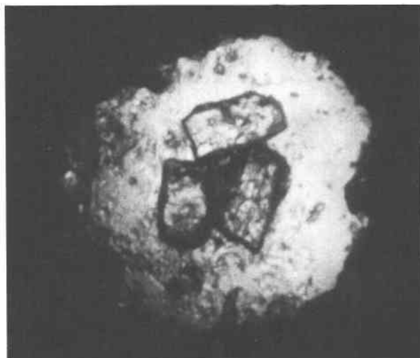
Fig. 1. Photomicrograph of three pyroxene crystals in diamond cell at 47 kbar. Diameter of the compressed gasket is approximately 300 μm.
