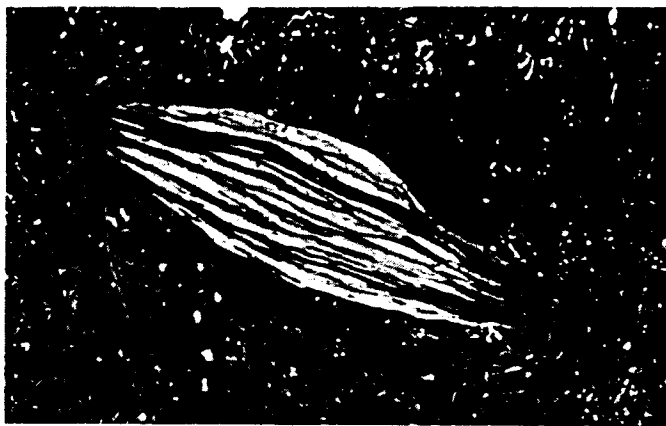
Fig. 3 BSE micrograph showing complex nature of interlayering in a chlorite-smectite stack. The delicate growth projection at the right-hand end of the stack is unlikely to have survived long-distance transport.
