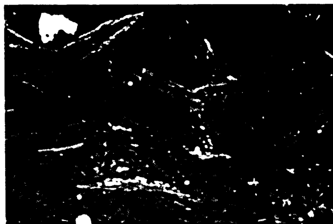
Fig. 4 BSE micrograph showing authigenic intergrowth of illite-smectite (I-S), kaolinite (K) and chlorite (C).
