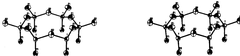
FIG. 6. Stereoscopic view of a portion of the annite tetrahedral layer, showing apparent thermal vibration ellipsoids. Orientation is as described in Figure 5.
