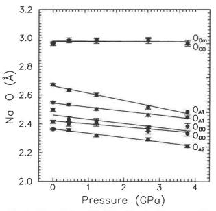
Fig. 5. The variation of Na-O bond length with pressure. The data are indicated by bars of 1 sd, and the lines represent leastsquares linear fits to the data. Note that only the five shortest bonds show any changes.
